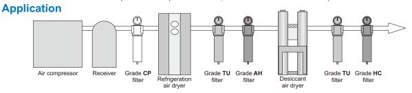
Note: 1. Grade TU filters after desiccant air dryer is for particle removal. Must be installed reversely and auto drain is unnecessary. 2. Grade HC filters is for oil vapor and odor removal. Auto drain and differential pressure gauge are not required.
